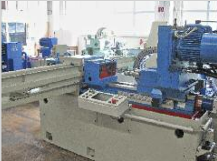
GKT M02-2-320 #573 Bohr/drill-Ø 2-18 mm, Bohrtiefe/drill depth 320 mm, Elektrik NEU/electric system and control NEW
