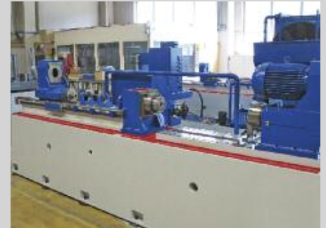
VENTURA V35-1000 #576 Bohr/drill-Ø 5-35 mm, Bohrtiefe/drill depth 1000 mm, Elektrik NEU/electric system and control NEW
