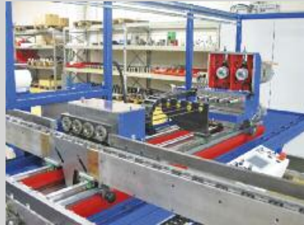
TIBO E15-4-750 #579 Bohr/drill-Ø 2-15 mm, Bohrtiefe/drill depth 750 mm, Neumaschine/NEW machine
