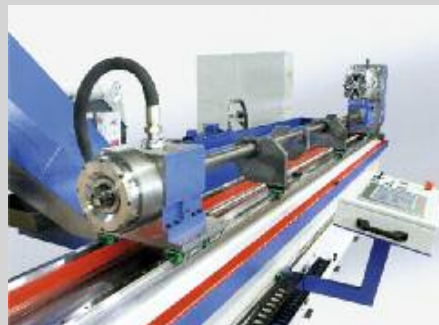
TIBO B65-3000 #548 Bohr/drill-Ø 18-65/100 mm, Bohrtiefe/drill depth 2550 mm, Reitstock/ tailstock, Neumaschine / New Machine
