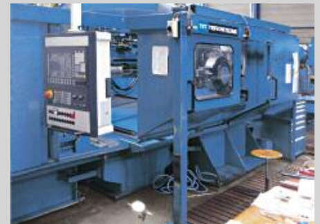
TBT BWP 250 #545 Bohr/drill-Ø -25 mm, Fräsen/milling, Spiral- bohren/spiral drills, Senken/tap, Gewinde- bohren/thread cutting, Siemens CNC 840D
