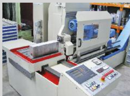
BS Flad KT #572 Bohr/drill-Ø 5-25 mm, Bohrtiefe/drill depth 500 mm, Kühlmittelanlage/coolant system NEW
