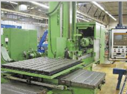
TBT/Collet T30-1000CNC #530 Bohr/drill-Ø 5-35 mm, Bohrtiefe/drill depth 1000 mm, Elektrik NEU/electric system and control NEW
