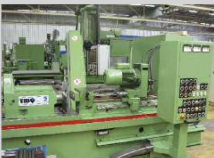
TBT T10-3-500 #506 Bohr/drill-Ø 2-7 mm, Bohrtiefe/drill depth 500 mm Taktband/loading belt
